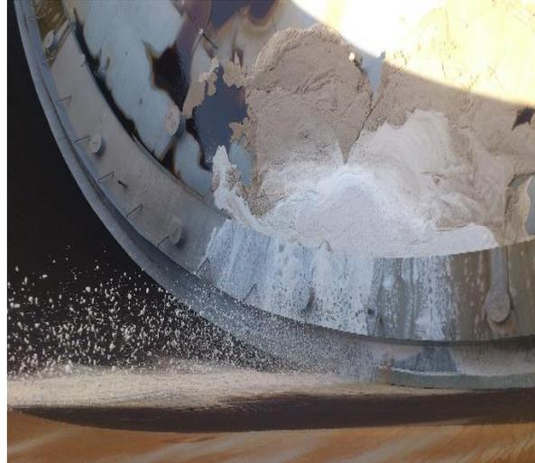
**Fig.3:** Excessive Foam Drainage from Foam Dam Causes Localized Foam Application
