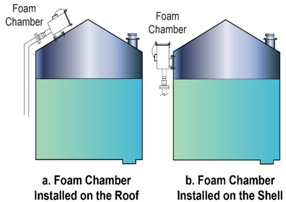
**Fig. 51:** Foam Chamber Installation for Fixed Roof Tanks
