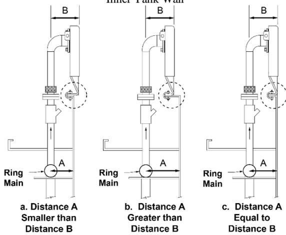
**Fig. 48:** Foam Pourer Installation on Top Angle
