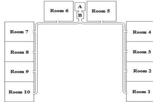
**Fig. 1:** Rooms plan and the air conditioner system (A: Water cooled air conditioner B: Silencer)
