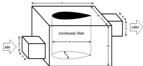
Fig. 3: The scheme of designed silencer
