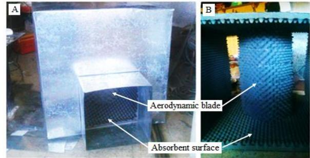
Fig. 5: Aerodynamic blade and absorbent surface outside (A) and inside (B) the silencer
