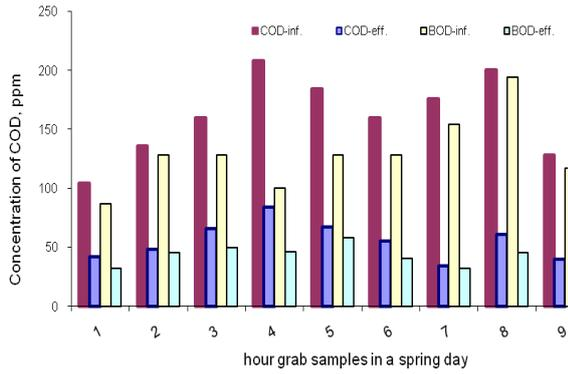
Fig. 6: COD and BOD<sub>5</sub> changes in influent and effluent in spring
