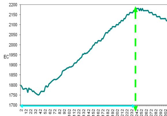
Fig. 4: Sample determination of optimum detection time by NaCl tracer method in high flow rate
