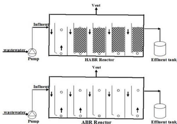
Fig. 1: schematic of the reactors
