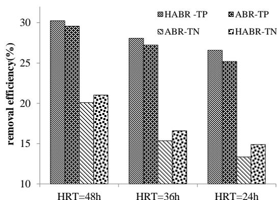
**Fig. 5:** Average TP (as PO<sub>4</sub>) and TN removals under steady state conditions
