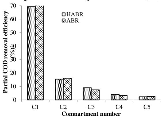
Fig. 2: COD removal in the various compartments of the ABR and HABR using a 36-hour HRT
