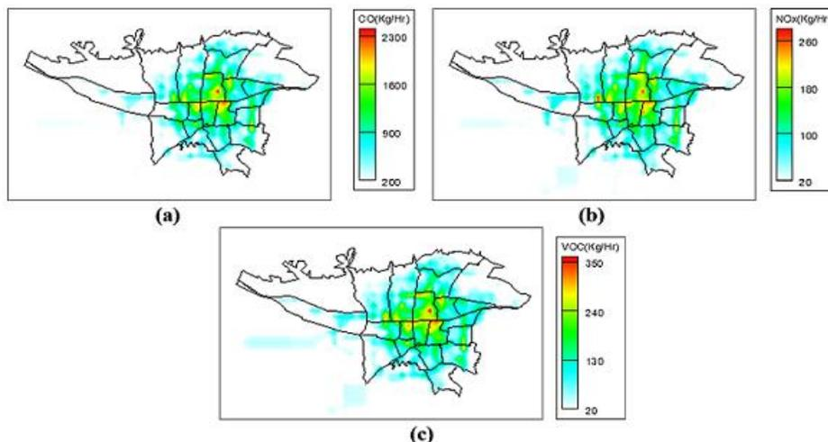
**Fig. 2:** Sample emission data for (a) CO, (b) NOx, and (c) VOC pollutants (kg/hr.) on the 1-km grid at 12:00 AM.
