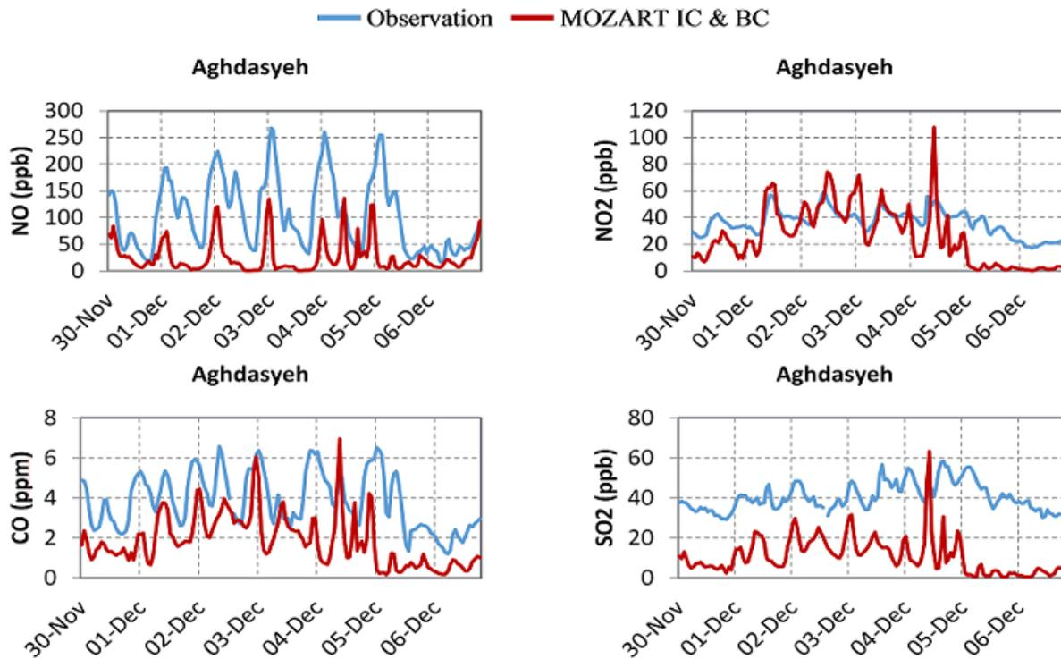
Fig. 6: Hourly time series of observed and predicted NO, NO<sub>2</sub>, CO and SO<sub>2</sub> concentrations at Aghdasyeh station, during November 30 to December 6. (— Observation — MOZART IC & BC)
