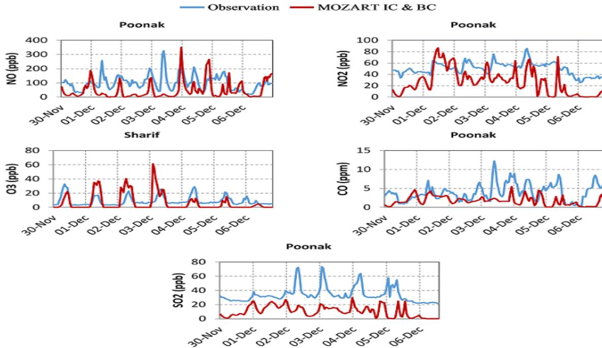
Fig. 5: Hourly time series of observed and predicted NO, NO<sub>2</sub>, CO and SO<sub>2</sub> concentrations at Poonak station and O<sub>3</sub> concentrations at Sharif station, during November 30 to December 6. (— Observation — MOZART IC & BC).
