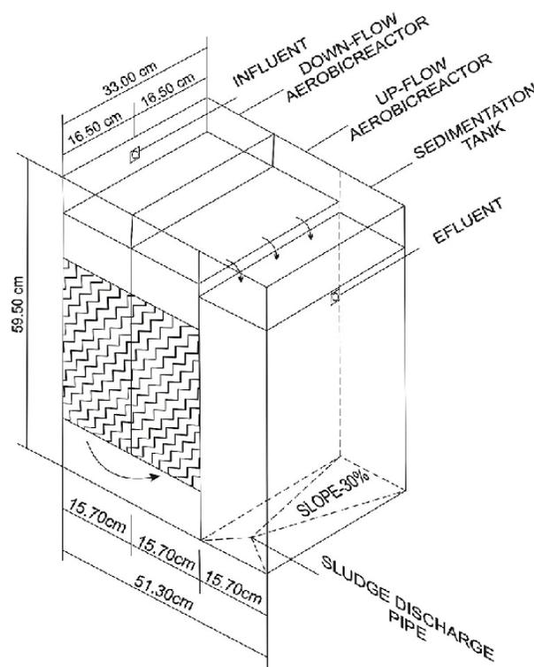
**Fig. 2:** Schematic diagrams of the IFAS system
