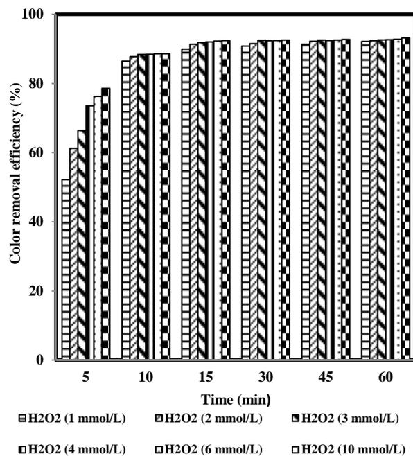
**Fig. 4:** Effect of H<sub>2</sub>O<sub>2</sub> concentration on the MB removal in the electro-Fenton process (experimental conditions: C<sub>0</sub>=100mg/L; pH= 3; applied current density= 1.4mA/cm<sup>2</sup>)
