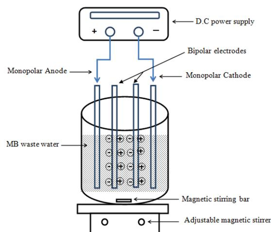
Fig.2: Schematic of electro-Fenton reactor with bipolar electrodes
