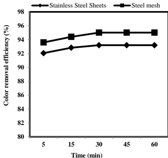
**Fig. 3:** Effect of electrode materials on the MB removal efficiency; C<sub>0</sub> = 100mg/L; pH = 3; applied current density= 1.4 mA/cm<sup>2</sup>
