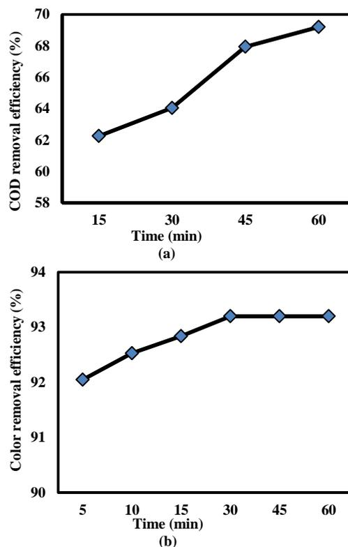
**Fig. 5:** Effect of reaction time on the (a) COD and (b) MB removal efficiency (experimental condition: C<sub>0</sub> = 100 mg/L; pH = 3; applied current density= 1.4 mA/cm<sup>2</sup>)
